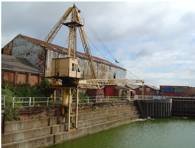
Fig.12 'Scotch' type derrick, Dock Office Row
